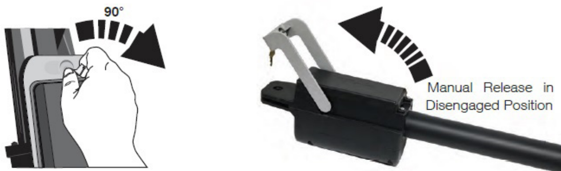
FIGURE 10-6 MANUAL RELEASE DISENGAGE
